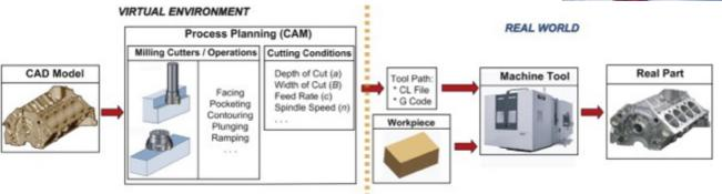
The aim of our research is to develop mathematical models of metal cutting operations, machine tool vibrations and control. The science based digital models allow the virtual design of machine tools, and testing and optimization of machining operations.
