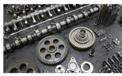
Some engine components requiring heat treatment
