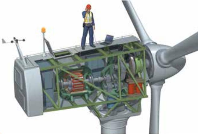
Gear mechanism in a wind turbine
