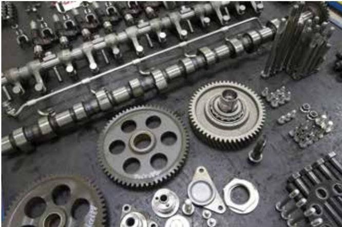
Some engine components requiring heat treatment
